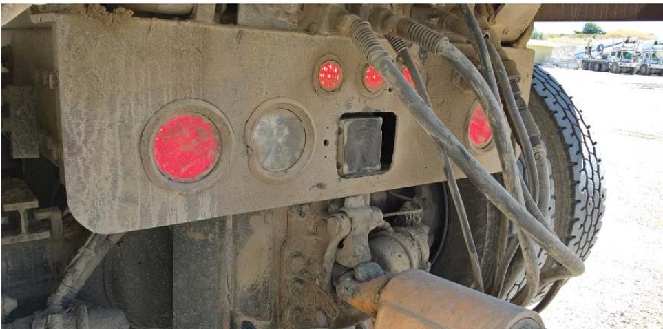
Above, a PRECO Electronics PreView Sentry sensor mounted on a hauler. (Photo: PRECO Electronics)
