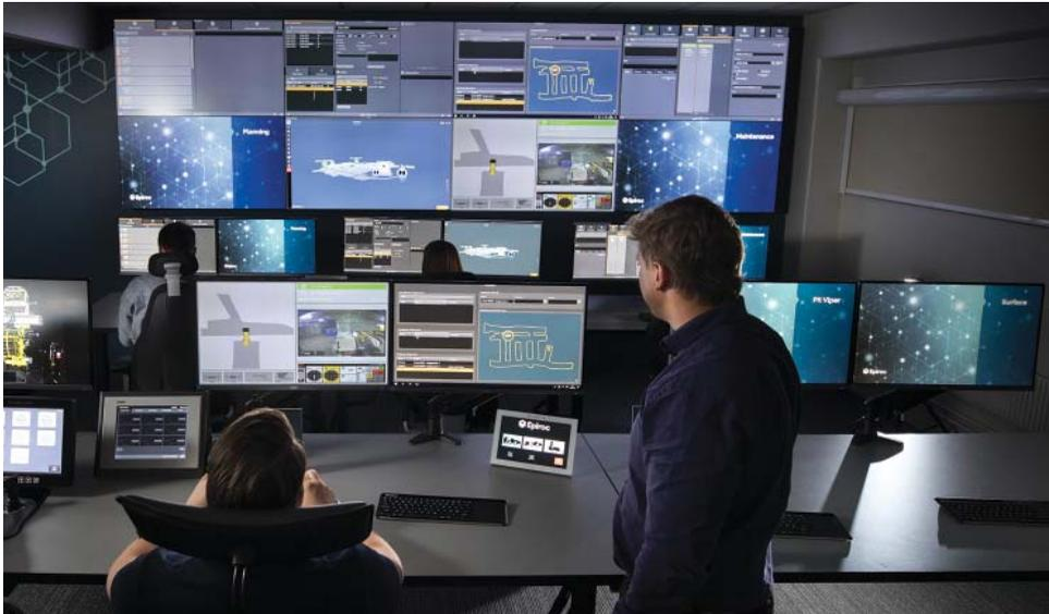
Fleet coordination in TMS is handled by a central node that uses data from an array of sources, a mine planning system, and a mine traffic control system. At the Epiroc Control Tower in Sweden, customers can explore and develop effective automation and information management solutions. (Image: Epiroc)
