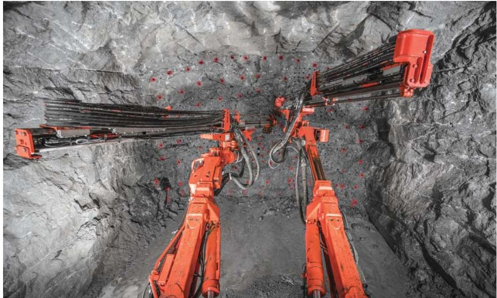
Above, an automation package will be offered later this year as an upgrade on two Sandvik development drills that will offer a boom collision avoidance capability. (Photo: Sandvik)
