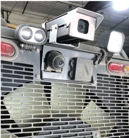
OmniPro Collision Avoidance System operates as a single-, dual- or three-camera system. Announced in November, it has been deployed to small mobile mining equipment and is currently being trialed on large trucks. (Photo: Matrix Team)
