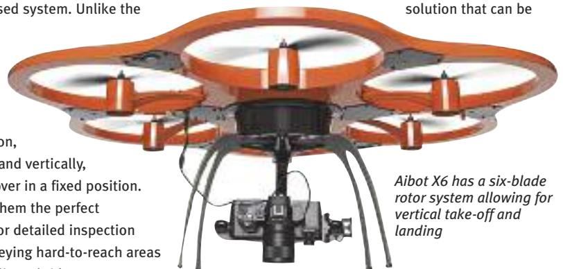
*Aibot X6 has a six-blade rotor system allowing for vertical take-off and landing*
