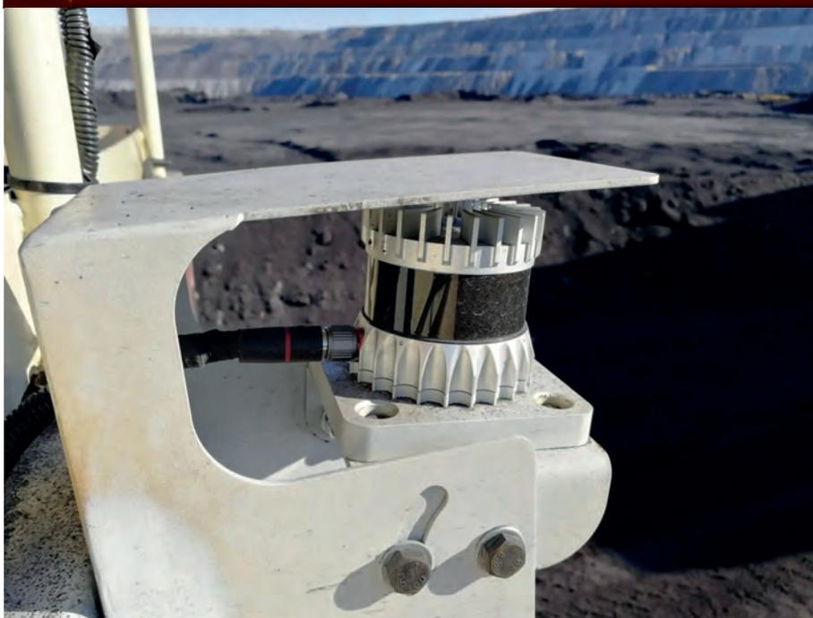
*Ouster LiDAR deployed on mining truck in China as part of automation solution from WAYTOUS*
