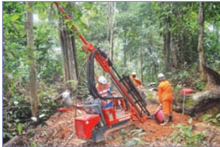
Dando Drilling's Terrier drill rig offers rotary drilling to 50m for a very low capital outlay
